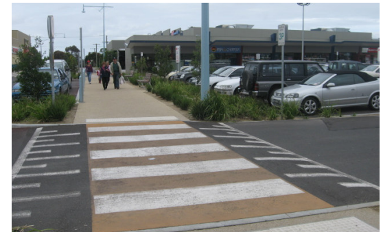
Raised tables such as the one above, will help to slow traffic and give more priority to pedestrians within car parking areas.
