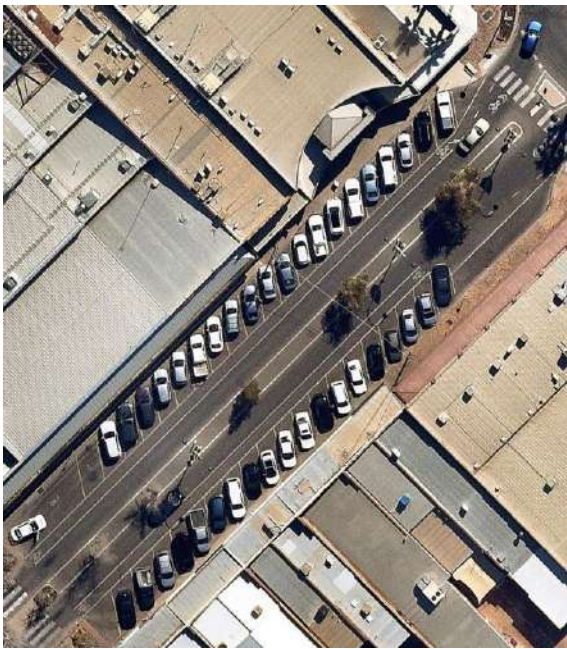
Figure 31 Poor line of site for vehicles reversing
