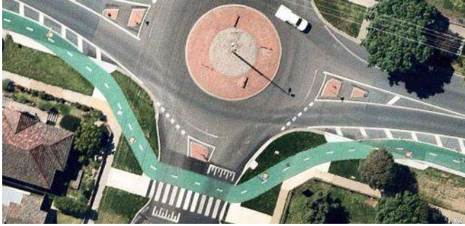
Figure 27 Protected roundabout, Bendigo
