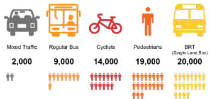
Figure 9 Carrying capacity of different modes, 3.5 metre carriageway
