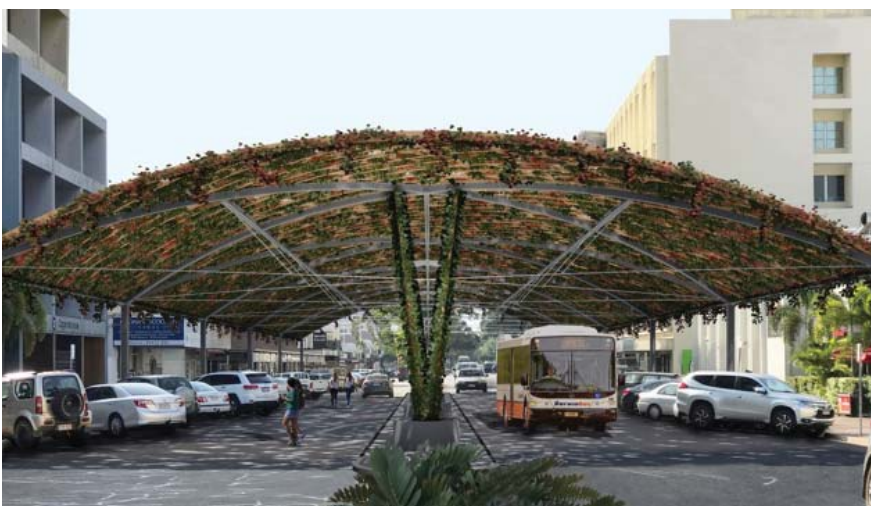
Image 51 Creative heat mitigation/shade canopy using vine planting (Cavenagh Street, Darwin - NT)
