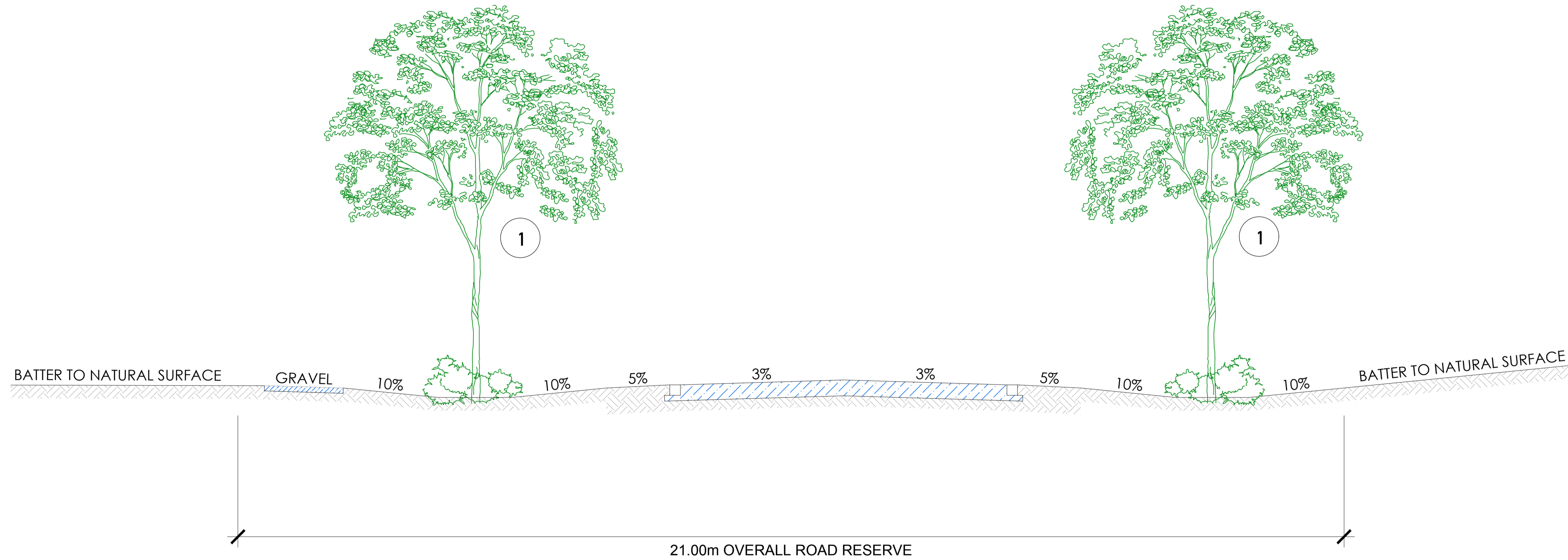
INTERNAL ROAD CROSS SECTION
