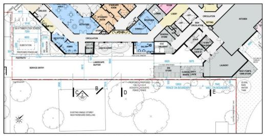
Figure 4 Noise barrier / fence documented within the architectural drawings
