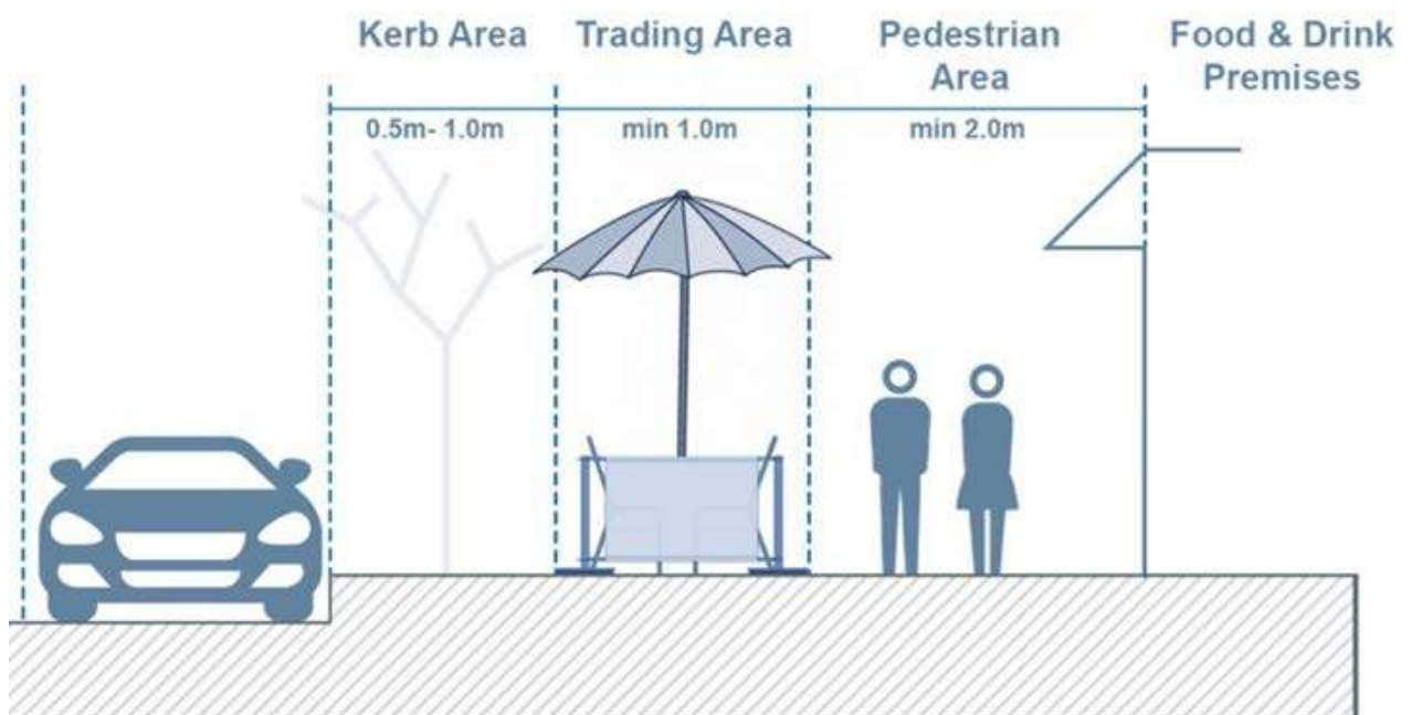
Figure 4 – Typical Section showing relative width of kerb depending on adjacent parking condition (Not to Scale)
